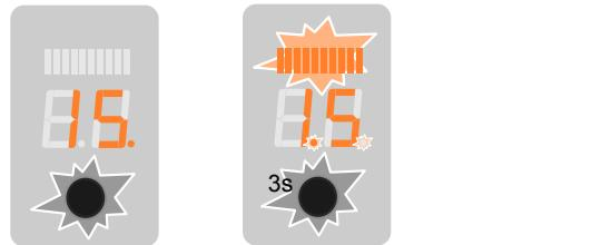
press button to reset flashing bar
